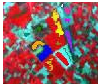
Fig. 2: Integrated false color image subset (97x82 pixels) with ROIs (training classes) of Mahtoli village and its nearby region by ASTER with a spatial resolution of 15 m per pixel.
