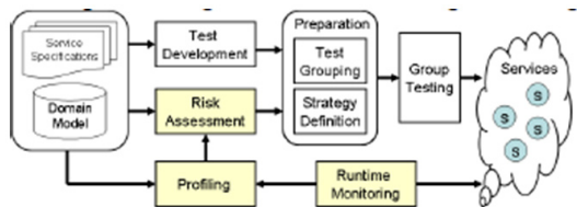
Fig.4: Adaptive testing of web based services
