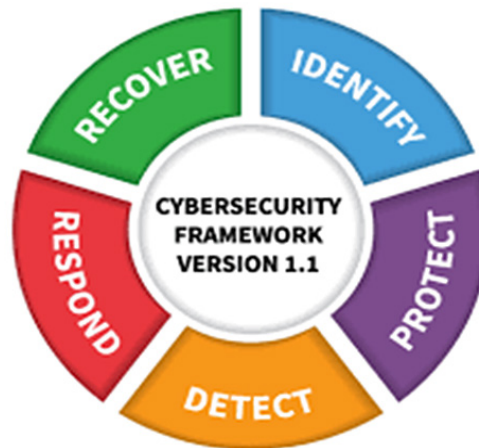
Fig. 4: NIST Cybersecurity Framework Core components. Source:National Institute of Standards and Technology 24
