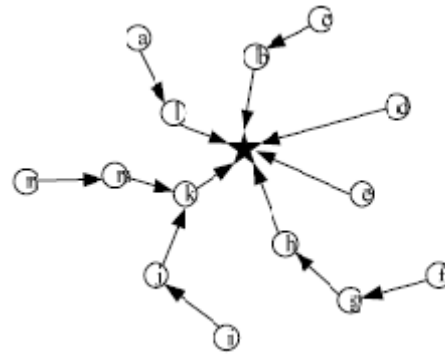
Fig. 2: Each node chooses its optimal multi-hop data transmission path to reduce energy dissipation
