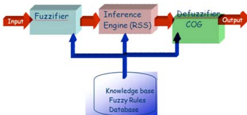
Fig. 1: The Architecture of Fuzzy Expert System for Malaria Diagnosis
